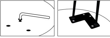
Use allen key(s) and threads to place and tighten screws.
