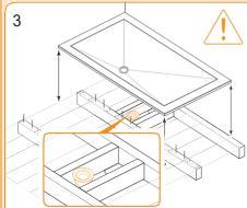
It is essential that the floor boards are properly secured, ensuring no movement orflex. Any joins in the floor boards that are not supported by a joist must be supported by separate noggin(s). Any floor boards that show flexing between joists MUST also be supported by additional noggin(s).
