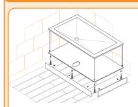
For more problematic plumbing situations, a comprehensive 'Fitting Kit' is available. This raises the tray off of the floor to provide a simpler plumbing solution. For further details, see your retailer or installer.
