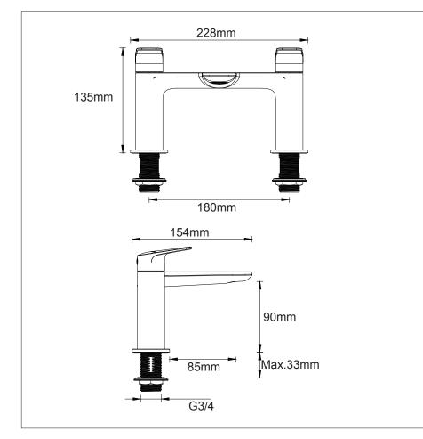
DIMENSIONS: ±5mm Width: 228mm Depth: 154mm Height: 135mm
