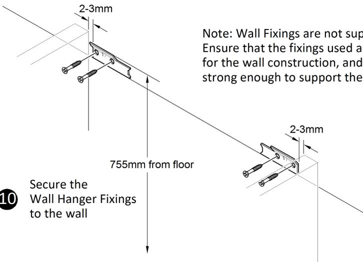
**10** Secure the Wall Hanger Fixings to the wall
