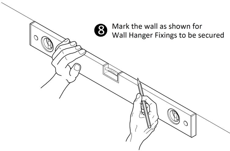
**8** Mark the wall as shown for Wall Hanger Fixings to be secured
