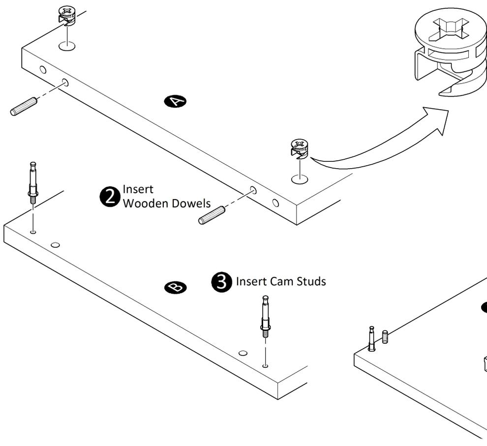
**1** Insert Cam Locks with arrow pointing towards the Stud Hole
