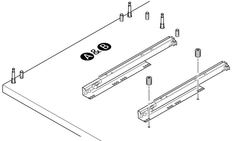
**4** Attach Drawer Runners x4 to both End Panels x2 with System Screws x8
