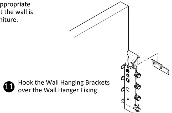
**11** Hook the Wall Hanging Brackets over the Wall Hanger Fixing
