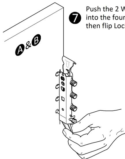
**7** Push the 2 Wall Hanging Brackets x2 into the four holes in each side Panel then flip Lock Tab down to secure
