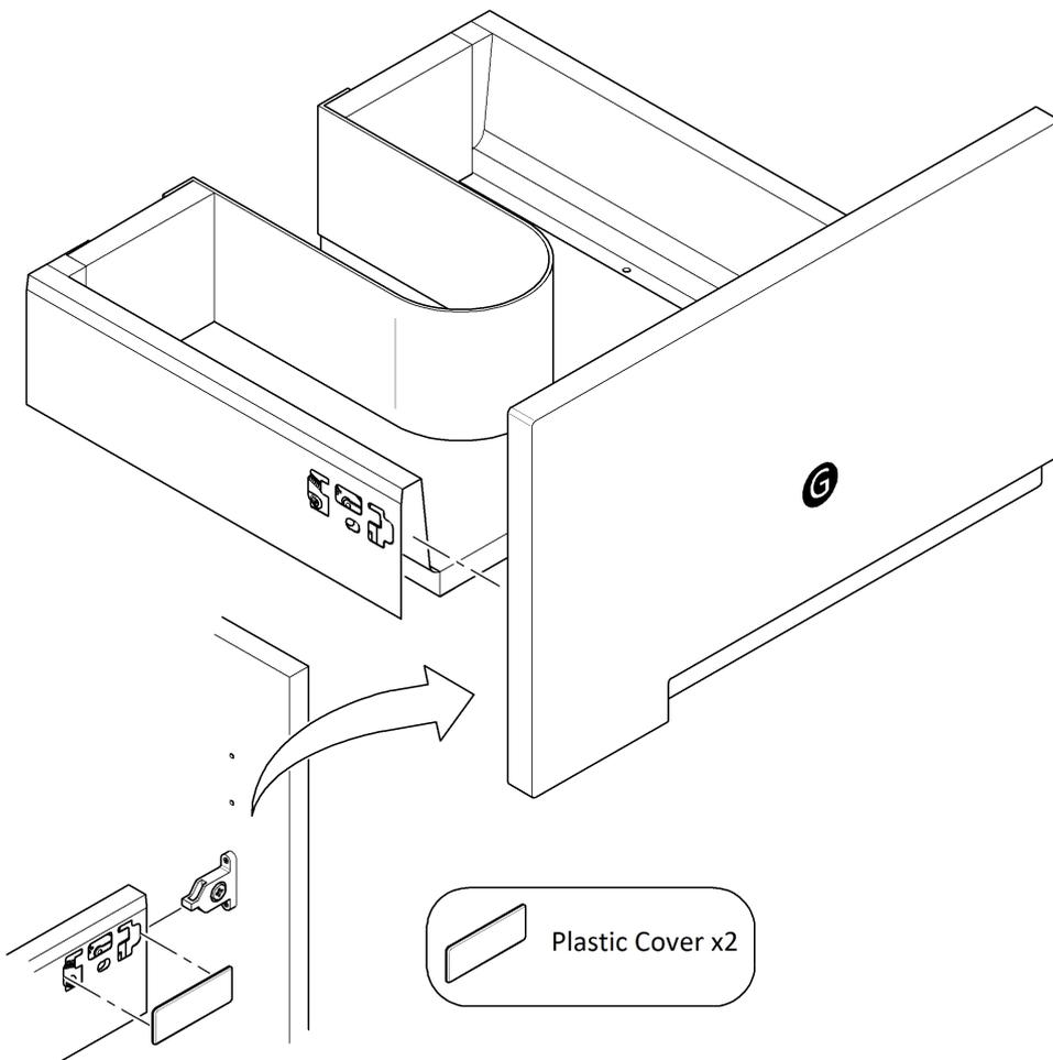
**16** Attach assembled Top Drawer components to Drawer Front
