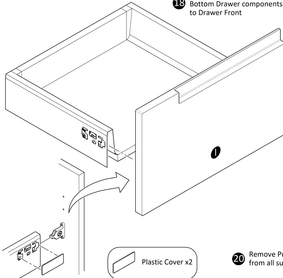
**19** When Drawer is assembled push Plastic Cover x2 into position
