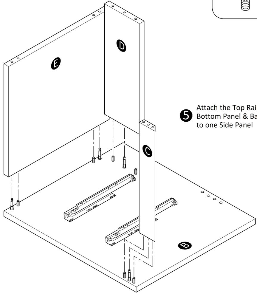
**5** Attach the Top Rail, Bottom Panel & Back Panel to one Side Panel
