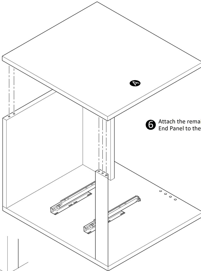
**6** Attach the remaining End Panel to the assembly
