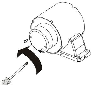
12. Using a screw driver, remove cable grip. Feed cable through hole & replace grip.
