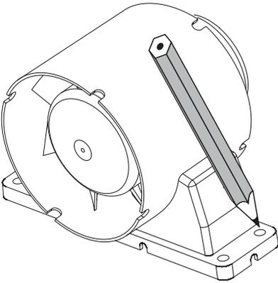
8. Fix motor to desired surface, using suitable wall plugs if necessary.
