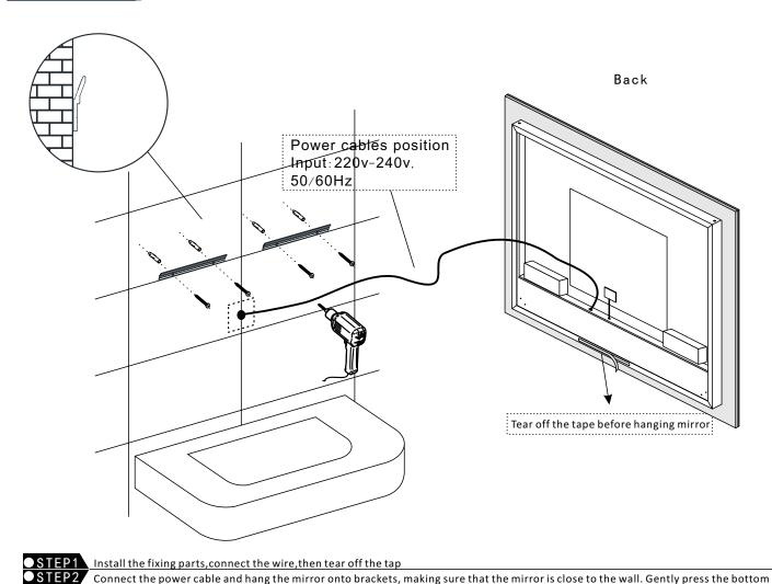
Connect the power cable and hang the mirror onto brackets, making sure that the mirror is close to the wall. Gently press the bottom of the mirror to ensure the double-sided adhesive touches the wall
