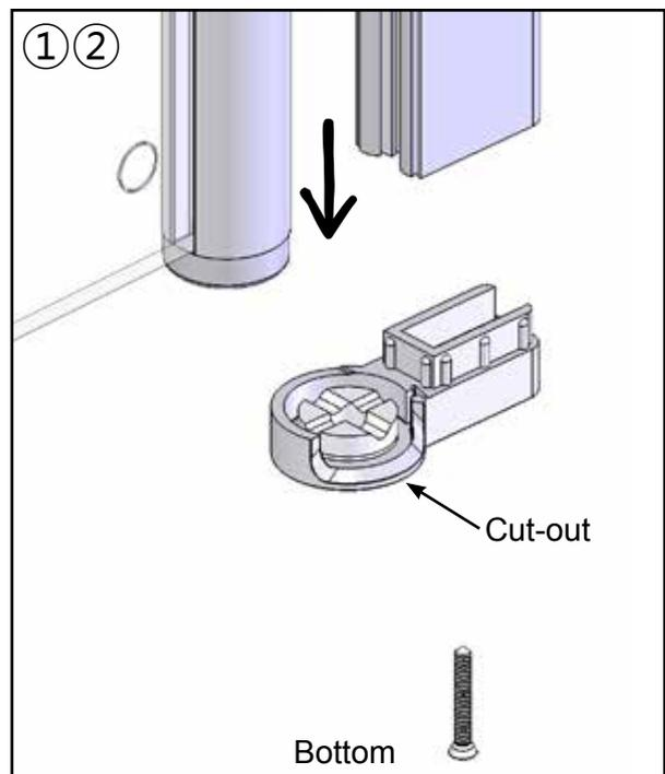
1. Place the Bottom Pivot Moulding into the Main Vertical Profile and secure using the No8 x 1½" Screw.
