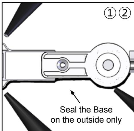
1. Using a Bath Room Sealant seal the Wall Profiles to the tiled walls both inside and outside vertically.
