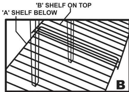
Shelves are fully adjustable and require no cutting. To adjust width, overlap the shelves making sure the shelf labelled A is placed first on the Brackets and the shelf labelled B is placed ON TOP of A.
