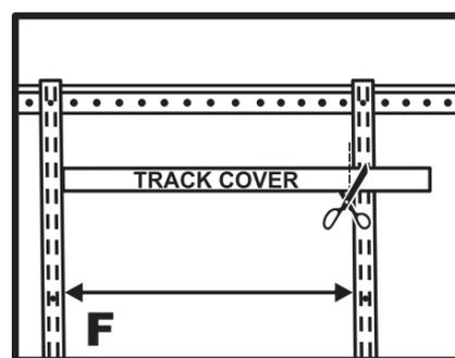
If the space between the last Wallstrip is less than the length of the Track Cover, you may choose to cut Track Cover with scissors to fit.
