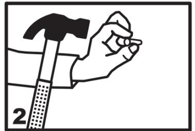
2 Hammer the wall anchor flush to the wall in the drilled hole.
