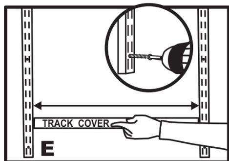
Hang another Wallstrip on the Track and use one of the Track Covers to space apart (ie 558mm). Drill a pilot hole and fasten screws in bottom hole of Wallstrip. (Use wall anchor if there is no stud). Place Track Cover over Track between Wallstrips. Repeat Step F for one or two more Wallstrips (if space allows).
