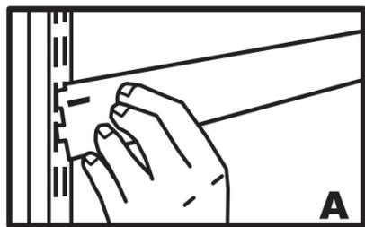
Insert Wire Shelf Brackets into Uprights at desired locations. **NOTE:** Install Wire Shelf Brackets and shelving at the top first and work down. Wire Shelf Brackets will not fit into upper slot of each Upright.
