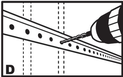
Starting at left side, fasten the FIRST TWO screws into studs (or anchors). Do not fasten remaining screws until after next step.
