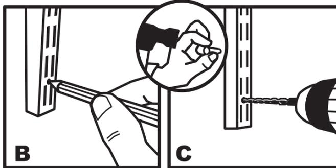
Mark bottom hole of Wallstrip. Drill a pilot hole into the stud (or wall anchor if no stud is available).
