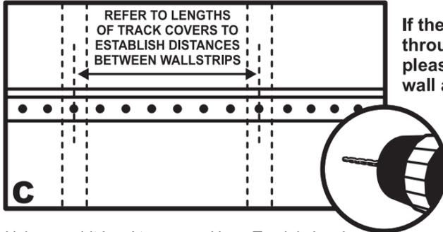
Using a spirit level to ensure Hang Track is level, mark the holes where the wall studs are, then drill a pilot hole.
