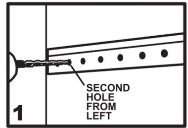
1 Mark and drill a hole (for a wall anchor) in the second Hang Track hole from the left.
