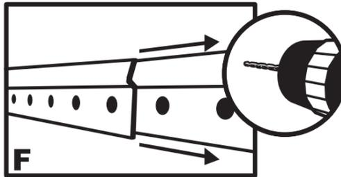
Slide second Hang Track to the right wall of the closet, and then back it away from the right wall until the holes in the two Tracks line up. Repeat Step C to secure to the wall.
