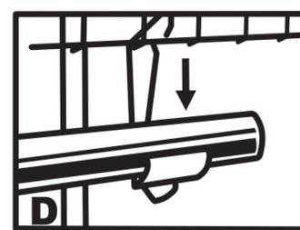
After expanding Clothes Rod to desired length, place into Hanging Rod Brackets and press down to snap into place.
