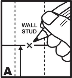
Locate all wall studs on closet wall and mark with an 'X' at the maximum height you require your system to be positioned.
