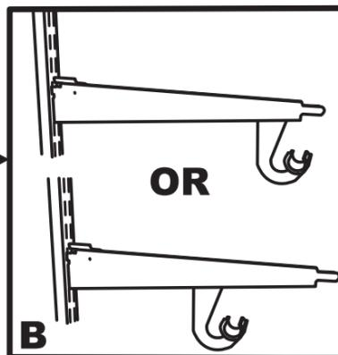
**NOTE:** Hanging Rod Bracket can be fixed to either of the 2 sets of slots in Wire Shelf Bracket, depending on depth of closet cavity.
