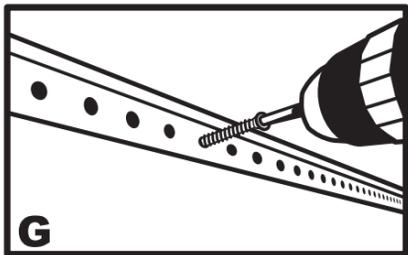
Install screws into studs (or anchors) along Hang Tracks
