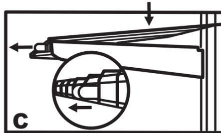
Make sure the Wire Shelf Bracket locks are unlocked (the plastic locking clip should be in a vertical position - upright) and install shelving making sure that the 'nose' of the Bracket is projecting out through the front edge of the shelf.
