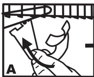
Install Hanging Rod Bracket into bottom of Bracket by tilting it backward until it locks in place.
