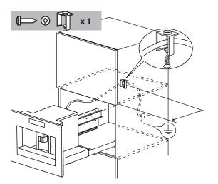
Position the machine on the runners, making sure that the pins engage properly in their seats before securing with the screws provided.
