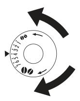
For slower run-off and creamier coffee, turn the knob I click in an anticlockwise direction (= finer ground coffee).
