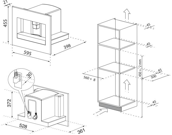
Position the runners on the sides of the housing, as shown in the Figure. Secure the runners with the screws supplied, then pull them out to full extension. If the coffee machine is installed above a "warmer drawer", use the top of the latter as a reference for positioning the runners. In this case, there will be no support surface.
