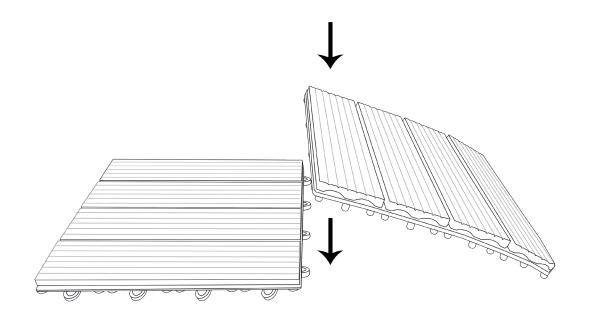
1. Composite deck tiles are vunerable to thermal expansion and will expand on all sides. Ensure a sufficient gap dependant on the size of area you are looking to cover is allowed for.
