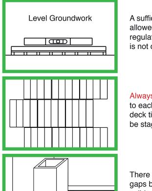
A sufficient gradient must be allowed for as per building regulations. Composite wood is not designed to sit in water.
